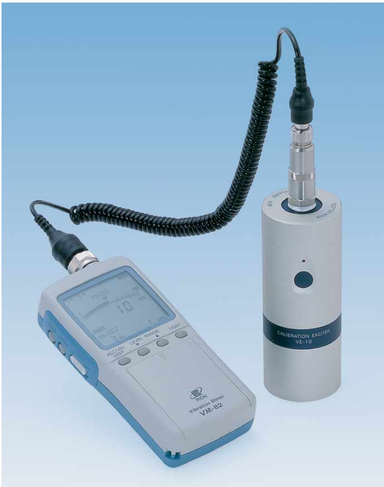
Calibration of Vibration Meter VM-82 by VE-10
